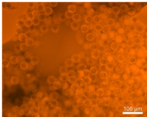
Figure S1: Fluorescent image of double emulsions after attempt for oil extraction with ethanol (24 h incubation, 28% ethanol in the outer fluid) as described in the literature [1]. Oleic Acid was stained with Nile Red.
